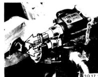
Pull off plugs on temperature switches.
