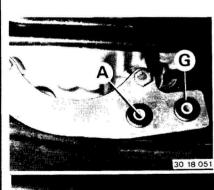
Push out spacers (A) and press out pivot sleeves (G). Installation: Coat pivot sleeves with a lubricant for installation of the spacers.
