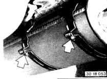
Loosen holder for final muffler. Installation: Torque\* holder in such a manner, that rubber
