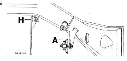
Tighten clamps (1) for the final muffler in such a manner, that rubber suspension parts are pre-loaded.
