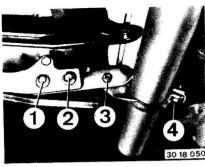
18 21 011 REPLACING PIVOT SLEEVES ON EXHAUST CARRIER
