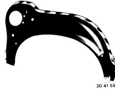
Grind mating surfaces on new wheel house
