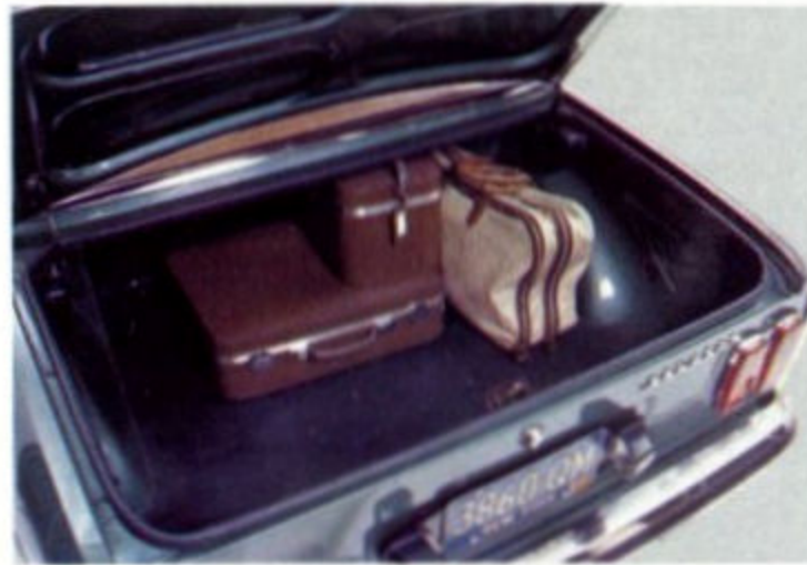
Big 15.7 cu. ft. trunk. More usable space because there's no spare tire to get in the way. And no need to unload baggage in case of a flat. Spare is stored underneath, locked in place from inside the trunk.
