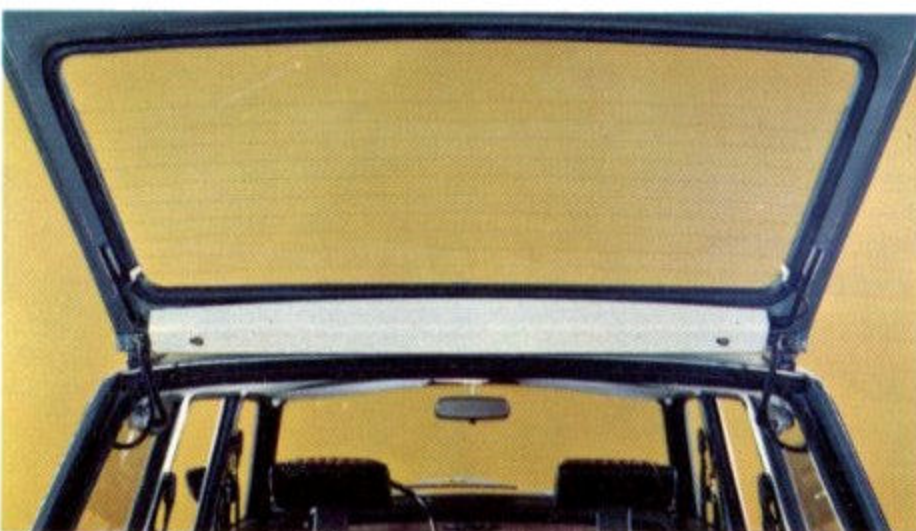
Door hinged at top for easy loading. Defroster clears rear window quickly.
